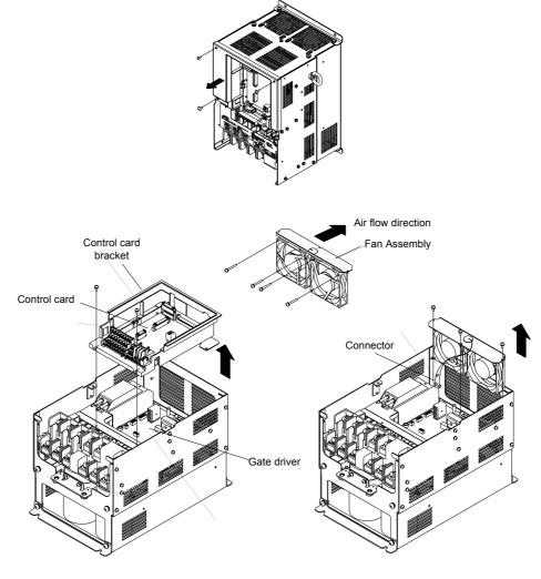
Fig 7.2 Cooling Fan Replacement (Inverters of 22 kW or More)
