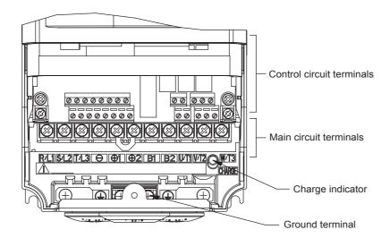
Fig 1.5 Terminal Arrangement (18.5 kW or Less)
