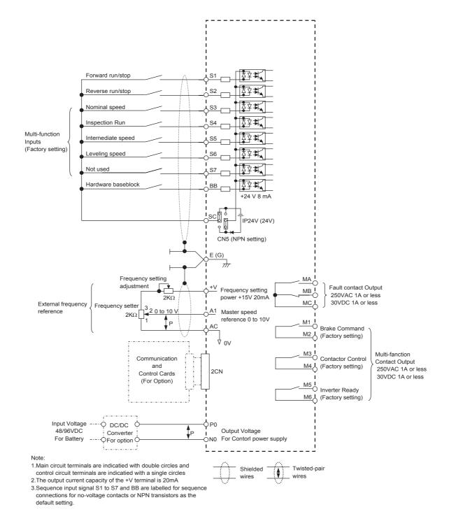
Fig 2.15 Control Circuit Terminal Connections
