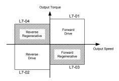
Fig 5.46 Torque Limit Parameters
