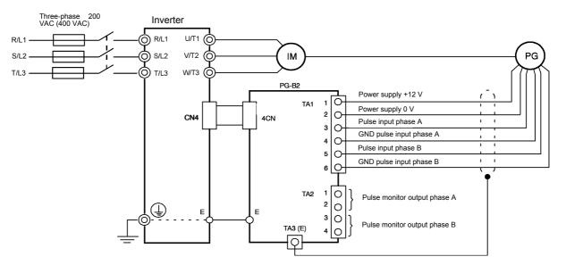
Fig 2.17 PG-B2 Wiring Using the Option Cards Power Supply
