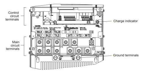
Fig 1.7 Terminal Arrangement (22 kW or More)
