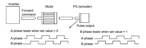
Example: Forward rotation of standard motor (PG)
