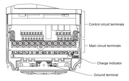
Fig 2.5 Terminal Arrangement (200 V/400 V Class Inverter of 3.7 kW)
