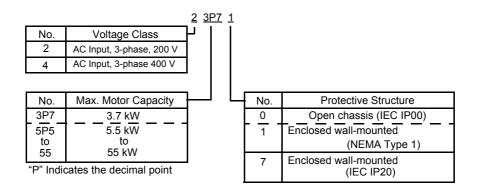
Fig 1.3 Inverter Specifications
