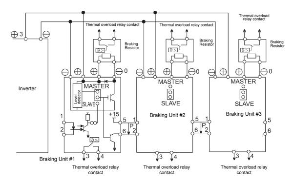
Fig 2.10 Connecting Braking Units in Parallel
