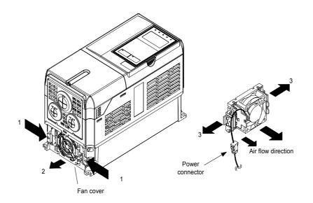
Fig 7.1 Cooling Fan Replacement (Inverters of 18.5 kW or Less)
