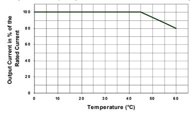
Fig 5.48 Ambient Temperature Derating Curve
