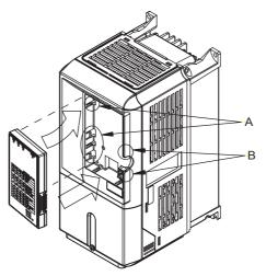
Fig 1.13 Mounting the Digital Operator/Monitor
