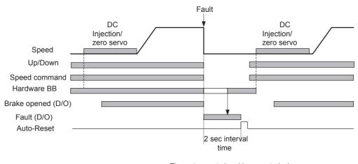
The auto-reset signal is accepted when the hardware base block signal is recieved .
