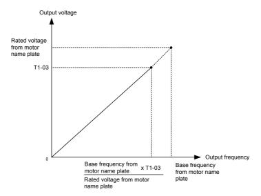
After the completion of autotuning, set E1-04 (Max. output frequency) to the base frequency from the motor's nameplate.
