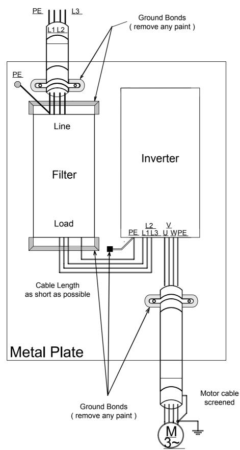
■ Installation inverters and EMC filters
