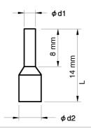
Fig 2.12 Straight Solderless Terminal Sizes
