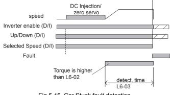
Fig 5.45 Car Stuck fault detection
