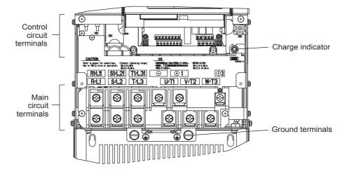
Fig 2.6 Terminal Arrangement (200 V/400 V Class Inverter of 22 kW or more)
