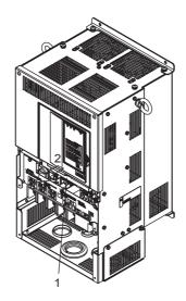
Fig 1.14 Removing the Front Cover (Model CIMR-L7Z4022 Shown Above)
