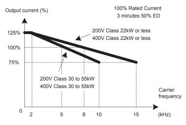
Fig 5.30 Current Derating depending on the carrier frequency
