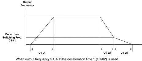
When output frequency < C1-11the deceleration time 4 (C1-02) is used.
