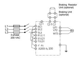
Control power is supplied internally from the DC bus at all inverter models.
