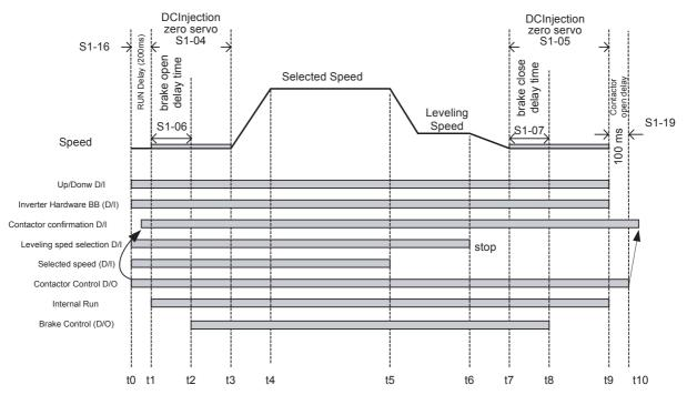
Fig 5.32 Timing chart of Brake sequence without torque compensation at start
