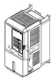
Fig 1.11 Removing the Digital Operator/Monitor (Model CIMR-L7Z43P7 Shown Above)
