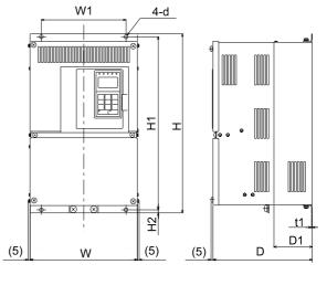
200 V Class Inverters of 22 or 55 kW 400 V Class Inverters of 22 to 55 kW
