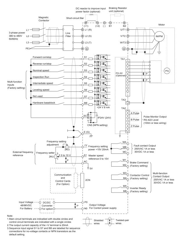
Fig 2.4 Connection Diagram (Model CIMR-L7Z43P7 Shown Above)
