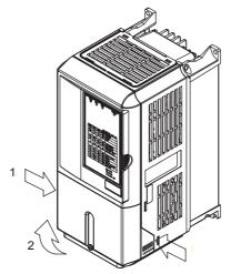
Fig 1.1 Removing the Terminal Cover (Model CIMR-L7Z43P7 Shown Above)
