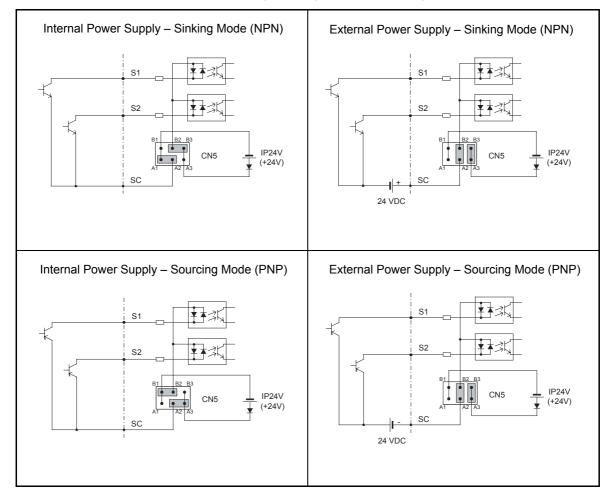
Table 2.11 Sinking/Sourcing Mode and Input Signals
