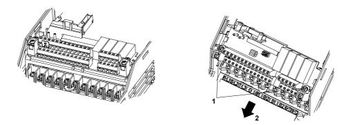
Fig 7.3 Removing the Control Circuit Terminal Card
