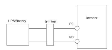
Fig 2.11 Connecting the battery power supply
