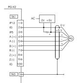
Fig 2.21 PG-X2 Wiring Using a 5 V External Power Supply
