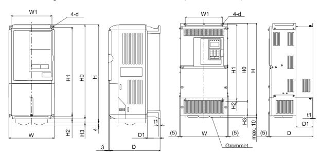
200 V/400 V Class Inverters of 3.7 to 18.5 kW
