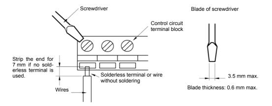
Fig 2.13 Connecting Wires to Terminal Block
